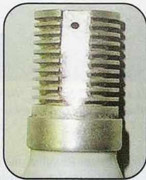
Photo 26. The GS-15B tube cooler is machined.
