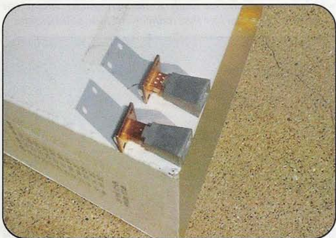
Photo B. Two more 15-dB gain horn antennas on the horn end of the large antenna in photo A. The big one covers the 2.3- and 3.4-GHz bands, while the little ones cover the 24-GHz band at the low end and 35 GHz at the high end.
