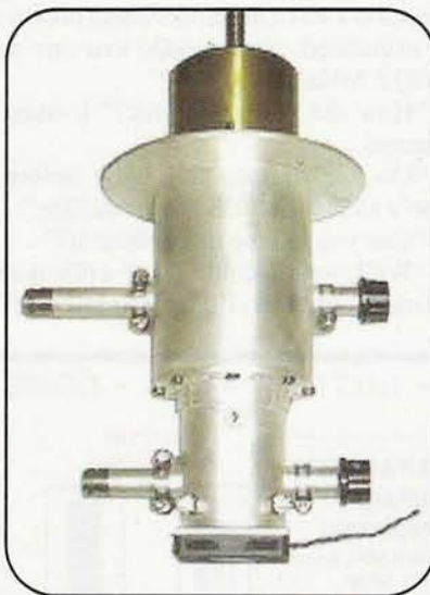
Photo 33. The KD5FZX 23-cm PA with water-cooled GS-23B installed.
