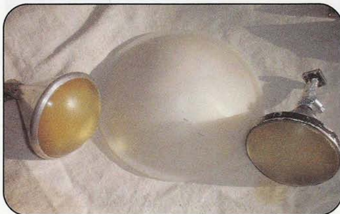
Photo F. This large lens, from a British 43-GHz horn-antenna system, was used to focus the waves into the receiver.
