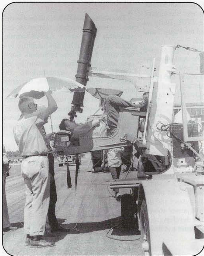
Forty-power binoculars for the pilot and a 50-power telescope for the "driver" were mounted on a gun mount for altitude record attempts at Dahlgren, Virginia on July 4 & 5, 1963.
