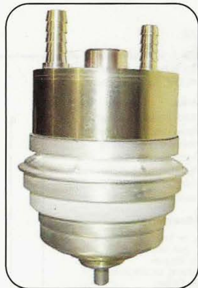
Photo 22. The GS-3A tube with the water jacket.
